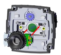
b. Tighten the M2 x 5 mm HSH screw halfway, then tighten the M2 x 12 mm HSH screw halfway as well. Continue screwing each screw incrementally, tightening them to 0.3 Nm using a torque wrench.
