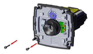
lacktriangledown Note: Start disassembling with unscrewing the M2 x 12 mm HSH screw on the left side. Continue unscrewing with the M2 x 5 mm HSH screw on the right side.
