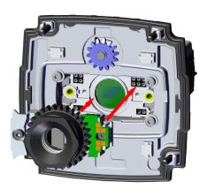
b. Tighten the the M2 x 5 mm HSH screw halfway, then tighten the M2 x 12 mm HSH screw halfway as well. Continue screwing each screw incrementally, tightening them to 0.3 Nm using a torque wrench.
