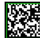
Quiet zone violation
